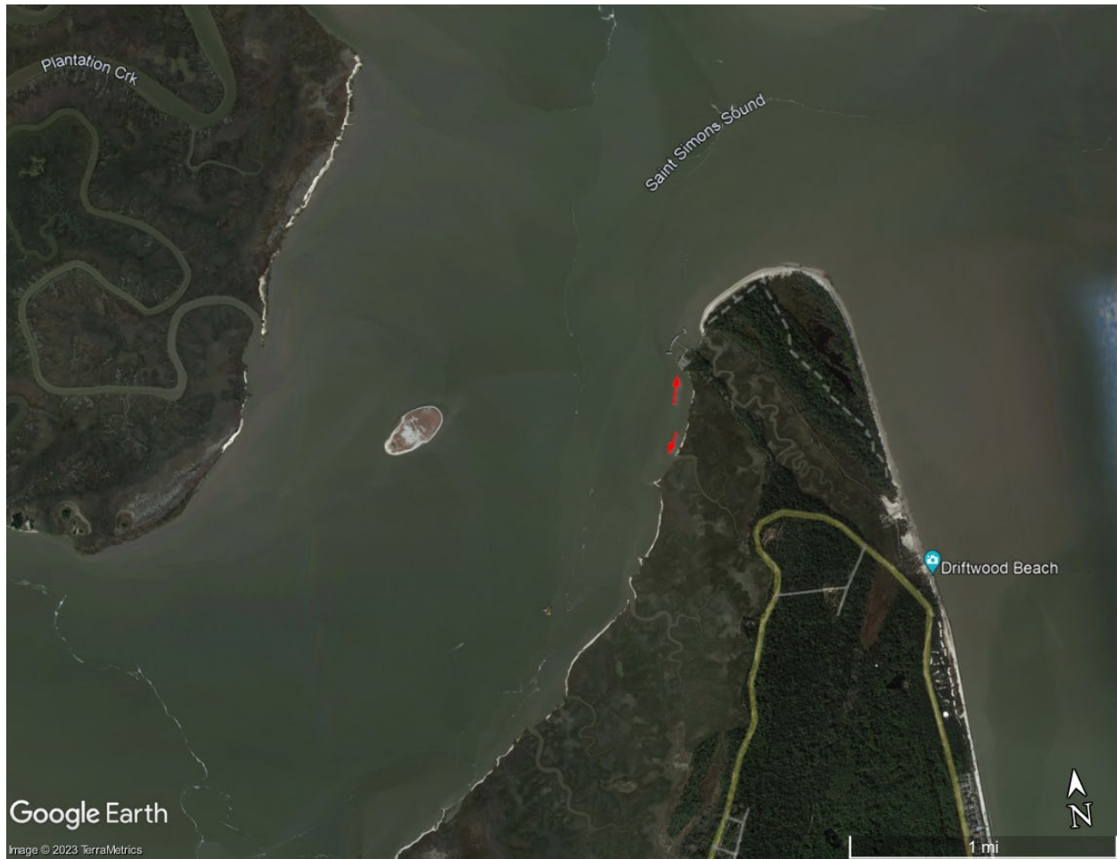
Figure 5. General turbidity plume directions at placement location during ebb and flood tides.
